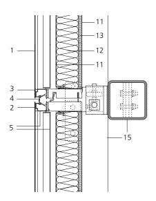
Vertical/horizontal section through façade panels scale 1:10
